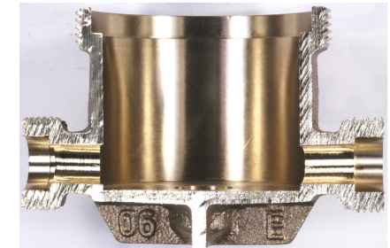
13mm bore Water meter
